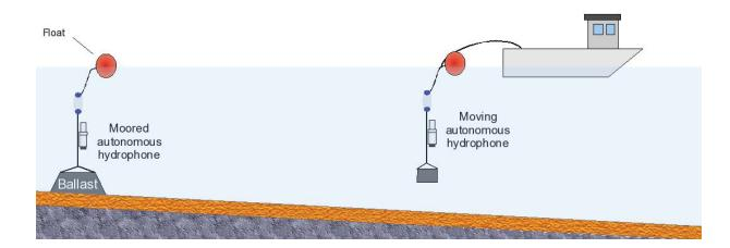
The digitalHyd SR-1 is powered by a rechargeable lithium-ion battery and is able to remain on for up to 10 hours of continous acquisition, or various days in stand-by. Battery and memory card are field replaceable, to allow for quick redeployments of the Hydrophone. Optional battery extension packs are available on demand, ex: the 4PACK option expanding the SR-1 to up-to 5x the autonomy.
