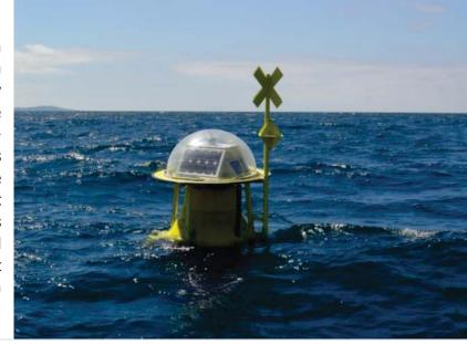
communication system (via GPRS or optionally via satellite), adding marine singnalling (mark, lantern and radar reflector). To complete the turn-key pack, customer may access data through Pagina Continuata Sensorum software pack, which includes graphics, tables and raw data without needing any installation at customer's computer systems.
